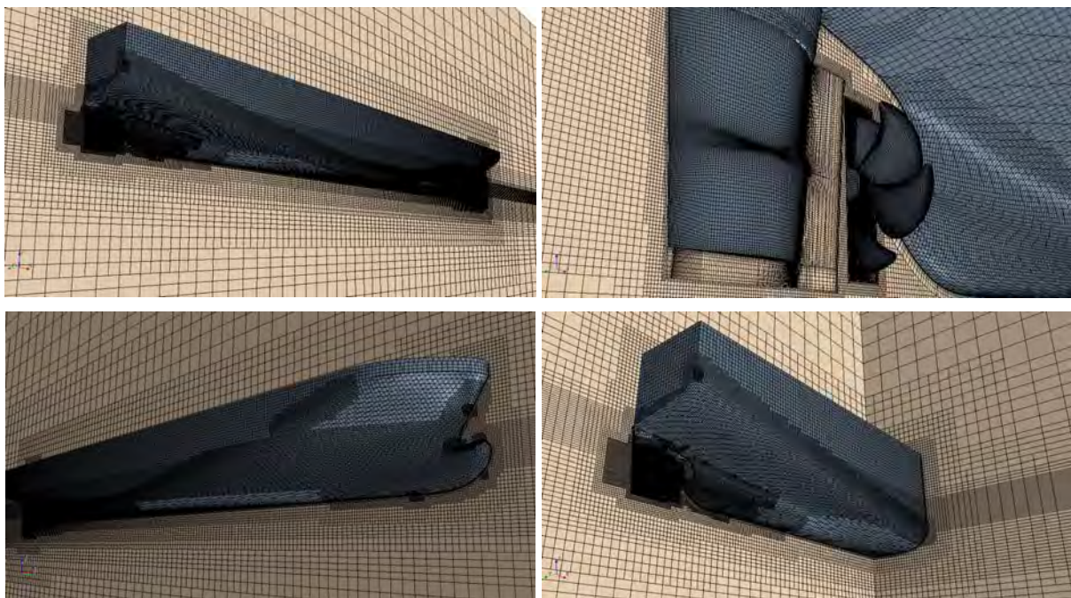
Figure 4: Computational grid around Container Vessel II, including views of rudder and propeller
