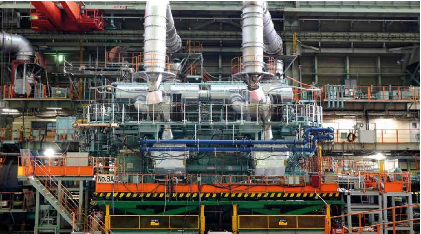
Schematic of the MAN B&W ME-GI two-stroke dual-fuel engine; designed for LNG/methane-powered vessels
