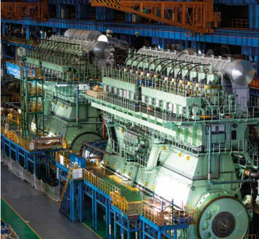
Schematic of the WinGD 12X92DF two-stroke dual-fuel engine; optimized for LNG and conventional fuel operation in marine vessels
