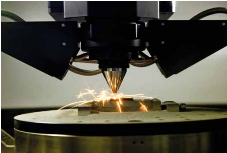
The Directed Energy Deposition (DED) process in action
