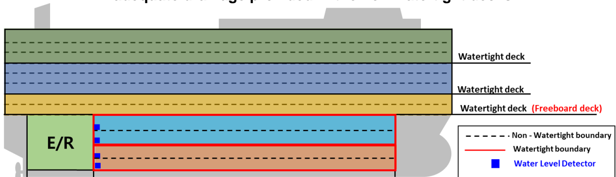
Figure 4: A multiple cargo hold ship with multiple holds below the freeboard deck with adequate drainage provided in the non-watertight decks
