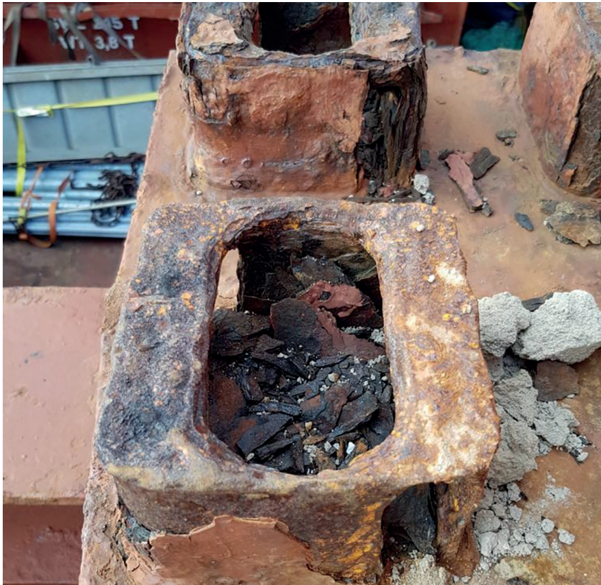
Figure 3 – IACS is developing Unified Requirement C8 to enhance the wear, tear, and corrosion of container stowage and securing systems
