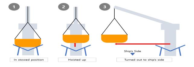
8 Based on the above illustration and the allowable launching appliance as per the LSA Code or the equivalency accepted by some flag State Administrations, IACS assesses the issue at hand as shown in the below table.
