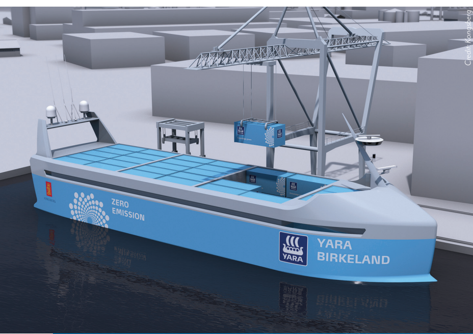
A computer generated image of the Yara Birkeland, the world's first crewless, fully electric and autonomous container ship
