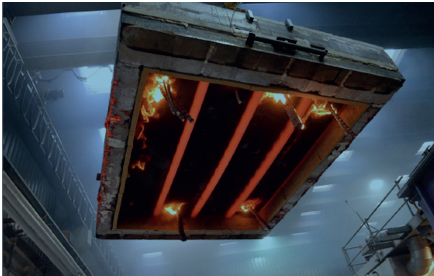
Fire test on deck cable penetrations, courtesy of Roxtec
