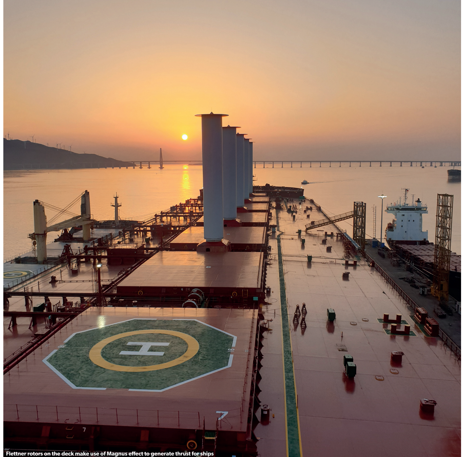
Flettner rotors on the deck make use of Magnus effect to generate thrust for ships
