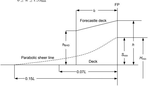
The height of the forecastle at the bulkhead position shall not be less than the ordinate, at that point, of a parabolic sheer curve having an ordinate  $S_{min}$  at the
