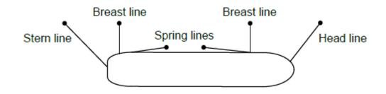
.4 Breast lines provide the maximum transverse restraint and spring lines the maximum longitudinal restraint against vessel movement in athwart and in fore- aft direction, respectively. Head and stern lines are much less effective for these purposes. The applied mooring layout should follow these principles as far as possible with respect to the port facilities and as far as reasonable with respect to the vertical line angles.
