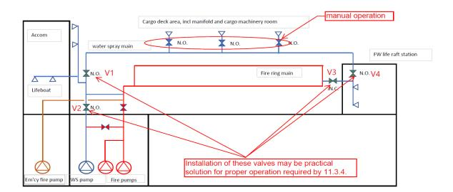
To illustrate the interpretation, the operation of the Normally Open (N.O.) valves V1 & V2 shall be arranged adjacent to the accommodation and V3 & V4 shall be arranged within the forward liferaft protected area.
